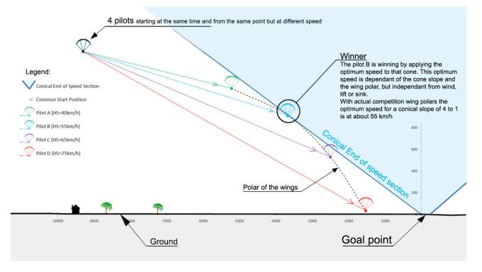
C) The first parameter of the new Competition Class is a limitation of the total available speed range of the Competition Class wings. At this stage PMA recommends setting a top speed limit of 65km/h, for the following reasons:
